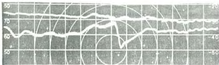
Fig. 5. Typical forward (upper) and reflected (lower) power at dipole inputs. 10 dB/div. Center frequency is 224 MHz.
