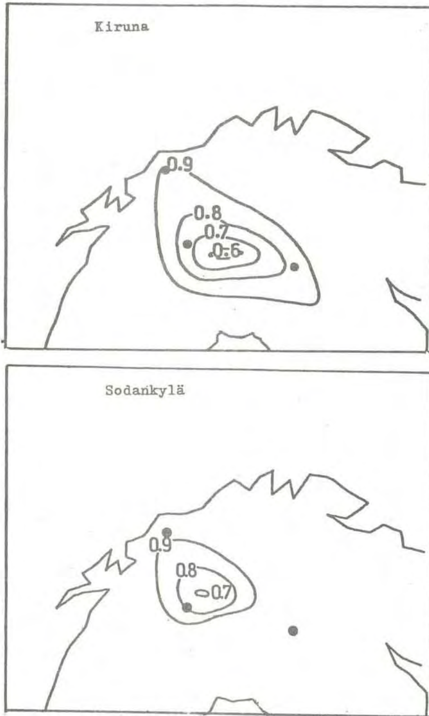
Figure 6.5 Relative powers received at Kiruna and Sodankylä when the polarizations are chosen to maximize the products of the powers received at the two stations. The computations refer to a height of 100 km (Murdin 1979)
