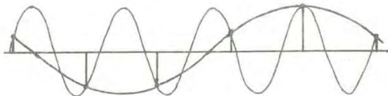
Figure 10.4 Sampling of sinusoid at \omega_s < 2\omega_e
