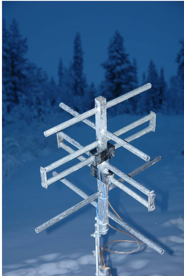
Figure 8.1.1: The first 235-MHz Renkwitz Yagi, constructed to the mechanical specifications given in Table 8.1.1 under typical midwinter conditions. In this beta version, the folded dipoles are made with movable shorting bars to allow a limited amount of fine-tuning. The production run antennas will have their dipoles made from formed continuous lengths of aluminium tubing. The blue cables that are strapped down onto the boom are half-wave baluns transforming the nominal 200 ohm balanced feedpoint impedance to 50 ohms unbalanced.
